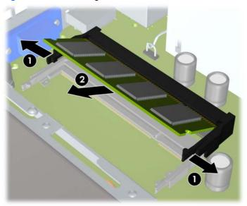
Figure 7-14 Removing a SODIMM
